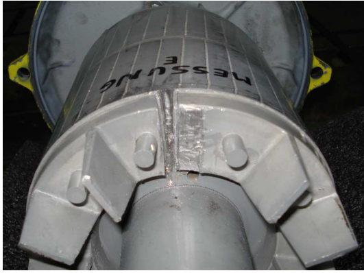
Figure 7: Squirrel cage rotor with respect to the configuration with one broken (removed) end ring segment
